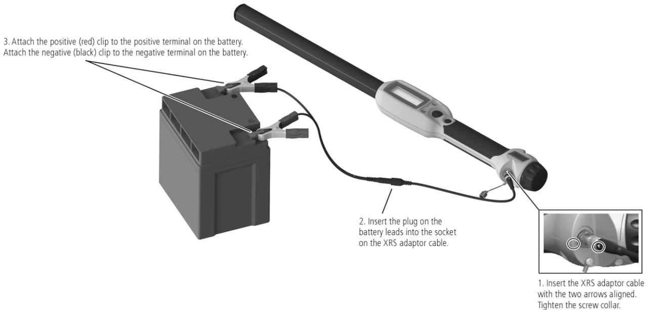
The stick reader may be used during battery charging, even if the battery is flat. To use the stick reader while the battery is charging, the internal battery must be in the battery compartment and the stick reader must be connected to the supplied mains power adaptor or a 12 V battery as described above.
